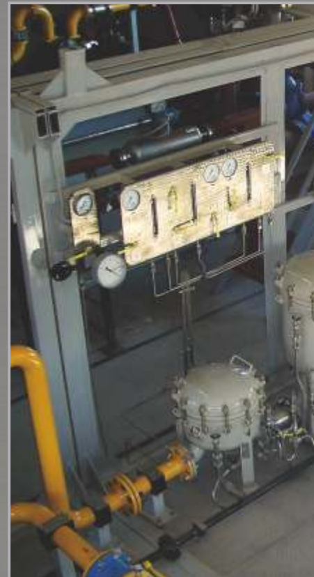
Fuel filtering unit AFT – 30-3-S (АФТ – 30-3-С) Function: feeding of CAFS, with triple filtration, eliminator in the fuel flow, and metering. Automatic control system
