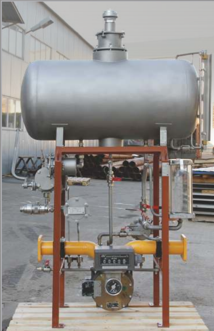
SD – 2290 (СД – 2290) Function: dosed injection of additives into the fuel.
