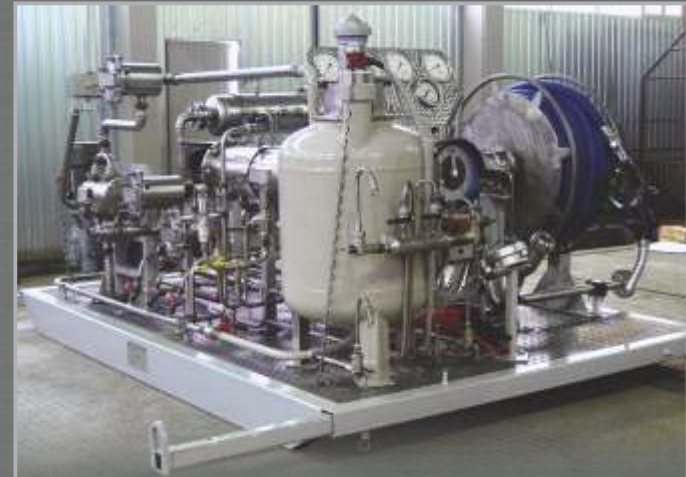
Fuel filtering unit AFT – 7-3-S (АФТ – 7-3-С) Stationary dispenser designed for aircraft filling with triple filtration, injection of liquids preventing water crystallization, and metering. Provides intake of aviation fuel and lubricants to the warehouse, pumping of fuel inside a warehouse, and loading of refueling trucks. Automatic control system
